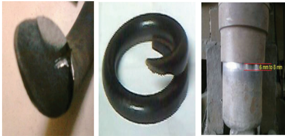
Fig. 13 Photographs of failed primary inner suspension spring and polished rubbing marks over damper
