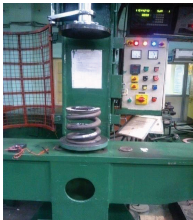
Fig. 2 Testing deflection of spring on spring testing machine
